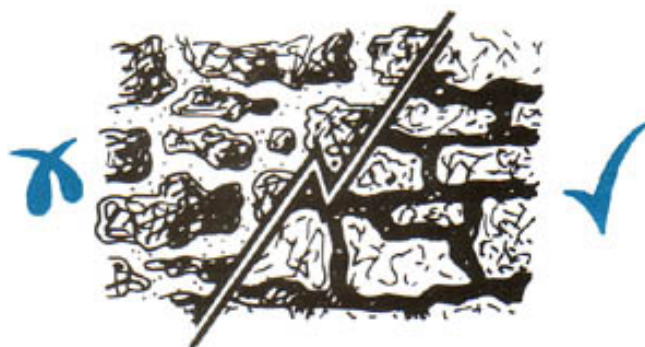
Suitable/unsuitable ways of repointing random coursed stonework
