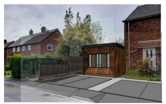
A new dynamic design has brought a change to the materials and external look of the new building, to reflect the 'green' construction use of a building system (Isotex) with its environmental accreditation. Largely finished with a clean render finish but with a front feature cladding in a brick coloured palette of sympathetic red/orange metal sheeting either to rust (corten steel) or a PPC corrugated sheet.
