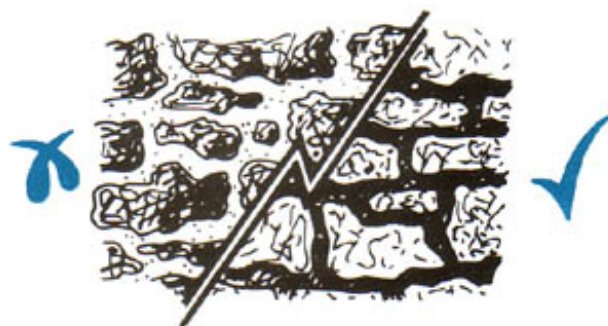
Suitable/unsuitable ways of repointing random coursed stonework
