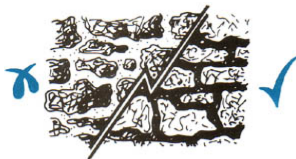
Suitable/unsuitable ways of repointing random coursed stonework
